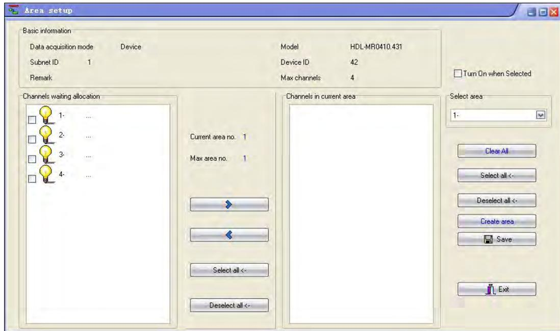
If the wiring required Channels 1 and 2 to be used to control 2 lights in a living room, and channels 3 and 4 to control 2 lights in the kitchen, the configuration process would be as follows:
