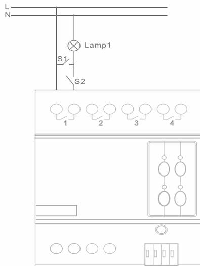
Turn on Lamp 1: Turn on S1, it does not matter if S2 is on or off.
