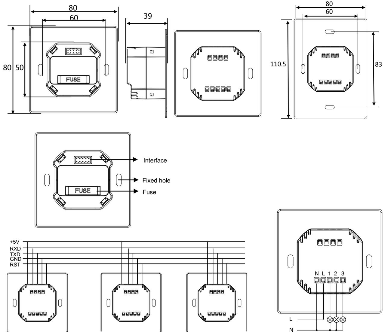
Multiple wireless power interface can be in parallel, then the panel (such as DLP) can control all channels. Shown as above, the terminal connection should avoid any mistakes.
