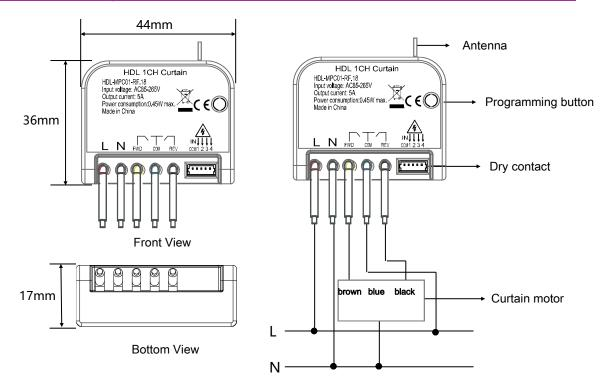
Programming button: if it is working properly, the green light will flicker, press the button three times continuously, the green light will flicker quickly, enter the setup mode (the gateway should enter the setup mode at the same time, and then, set the parameter)
