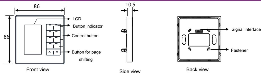
**Button Indicator:** Indicates the status of the target. On – Status on, Off – Status off.
