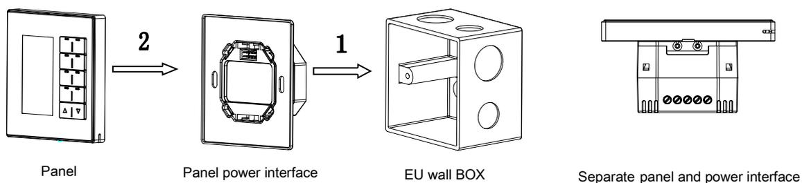
**Installation:** Hold the edge of panel, insert the power interface module vertically. Do not push the panel too hard.
