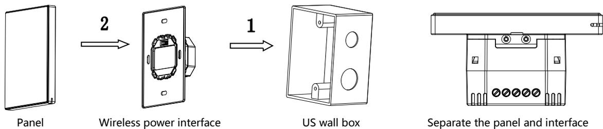
**Installation:** Hold the edge of panel insert the power interface module vertically.
