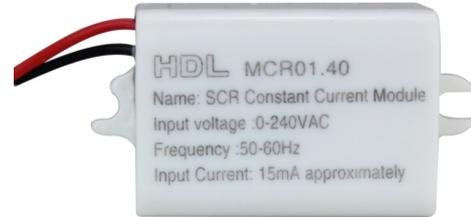
**HDL-MCR01.40** is a TRIAC constant current load, the module can supply minimum current for TRIAC. It can solve the flicker problem when it is dimming the lamps, such as LEDs and electronic transformer.
