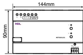
2CH 3A MOSFET Dimming Actuator
