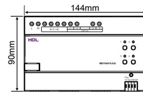
4CH 1.5A MOSFET Dimming Actuator
