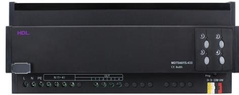
**HDL-MDT04015.433** Dimmer is based on the technology of MOSFET. It has 4 output channels and manual switch is available for each channel. Each channel can choose leading edge or trailing edge by software. This is very useful when user has different type of loads. And it has short circuit protection and over heat protection
