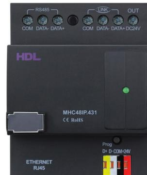
**HDL-MHC48IP.431** Hotel room control host which is the core of the hotel system, it can work in conjunction with mix controller. Hotel control host has 48 channels, it must be set from hotel management system. Hotel management software can set the parameters for system, control and monitor doorbell panel, curtain, lights, fan and A/C.
