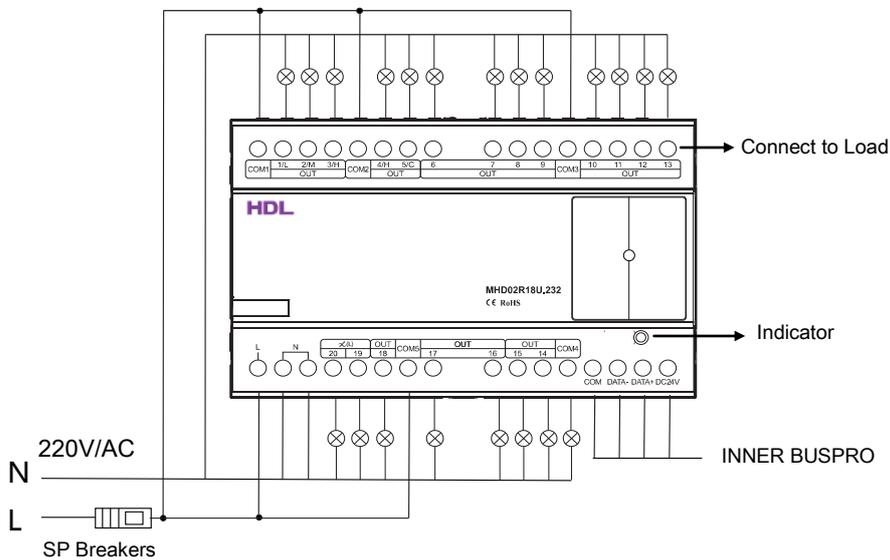
**Indicator:** flickers when the module is working properly. Keep pressing for 3 seconds, it can be read and modify the start address in the HDL-Hotel Room Intelligent System Manage Software.
