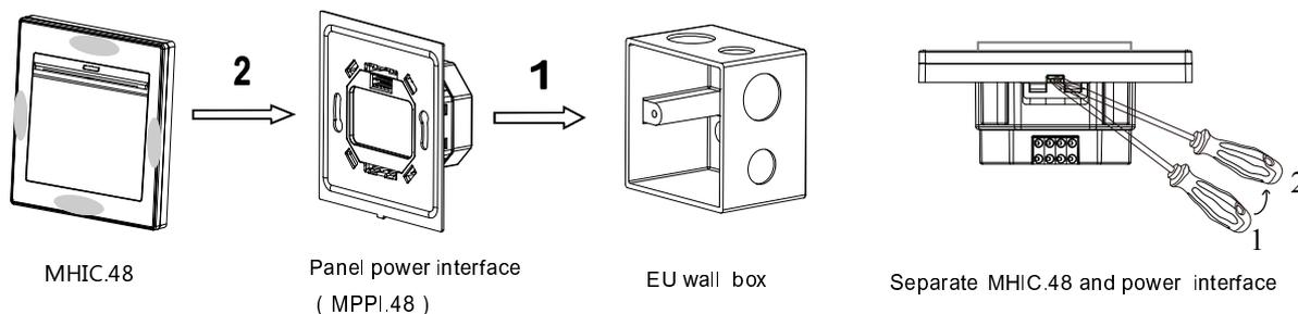
**Installation:** Hold the edge of MHIC.48 (shown as above), insert the power interface module vertically. Do not push this module too hard.
