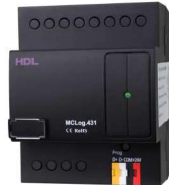
HDL-MCLog.431 is the HDL Logic Module. It has 960 Logic blocks, and the inputs condition of logic can be set scene status, channel status, date, week, time, external input value, external input status etc. By using different logic relations to set up different control target. 4 Logic relations are available for each logic block: AND, OR, NAND, NOR .
