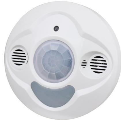
**HDL-MS12.2C** 12 in 1 sensor includes temperature sensor, PIR motion sensor, LUX sensor, ultrasonic sensor, dry contacts, IR received, IR emitter, 2-channel 5A relay output and logic block. The logic block can combine all sensors for different applications. It supports HDL security mode and command.
