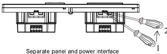
**Split:** Insert a 2.5mm-screwdriver to the split gap, pry up from position 1 to 2, wiring hole will open. Then separate the panel and MPPI.48.
