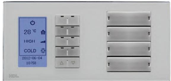
**HDL-MPL8.48** 8-button multifunction LCD switch is a new generation of wall-mounted switch with new design. It has 8 control buttons and the left & right side of the button can be programmed separately. There are 2 buttons are used for the page switching. Each button can display an icon in the LCD screen and the icon can be customized for final user.
