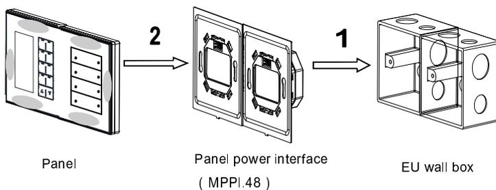
**Installation:** Hold the edge of panel, (see pictures on the left), insert the power interface module vertically. Do not push the panel too hard.
