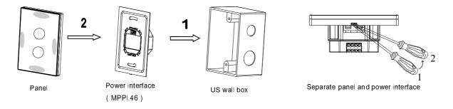
Installation: Hold the edge of panel (shown as above), insert the power interface module (MPPI.46) vertically. Do not push the panel too hard.
