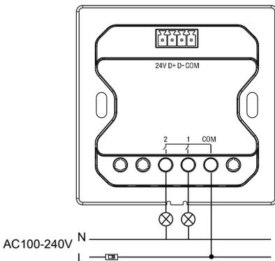
Figure 7. Wiring
