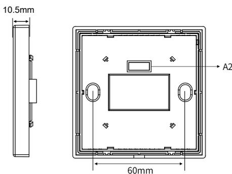
Figure 4. Dimensions - Side View Figure 5. Dimensions - Back View
