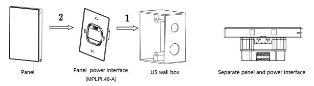
Installation: Hold the edge of panel (shown as above), insert the power interface module vertically.
