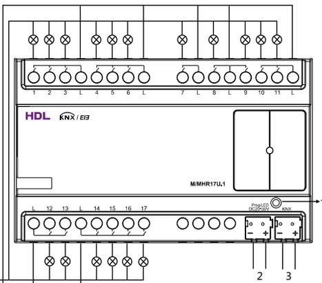
Figure 4. Wiring
