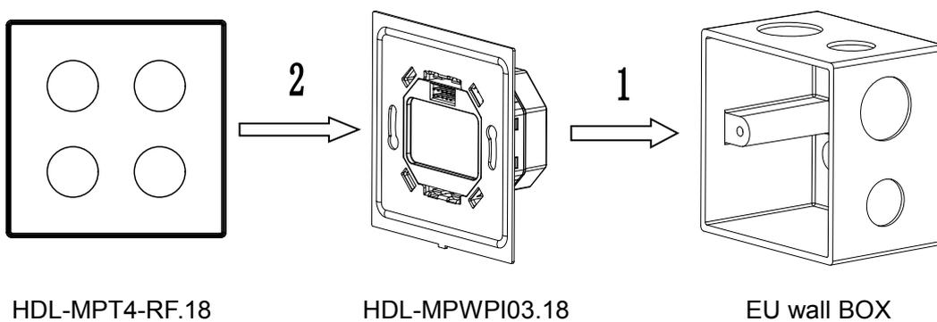
Separation: Use a screwdriver with 2.5mm insert to split gap, pry up, from position 1 to position 2, the wiring hole will open. Then separate the panel and power interface.
