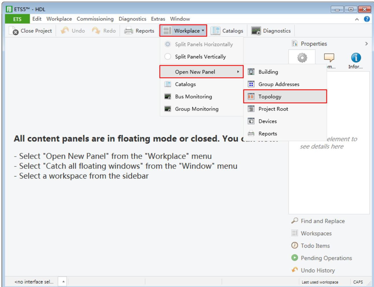
Figure 1-7 Open configuration window
