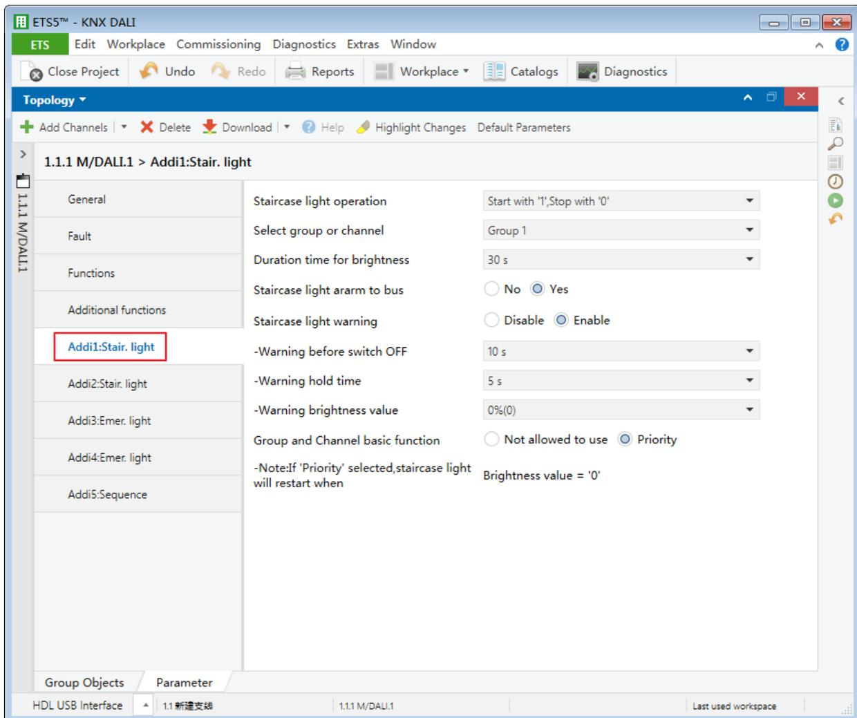
Figure 8-2 Staircase light setting
