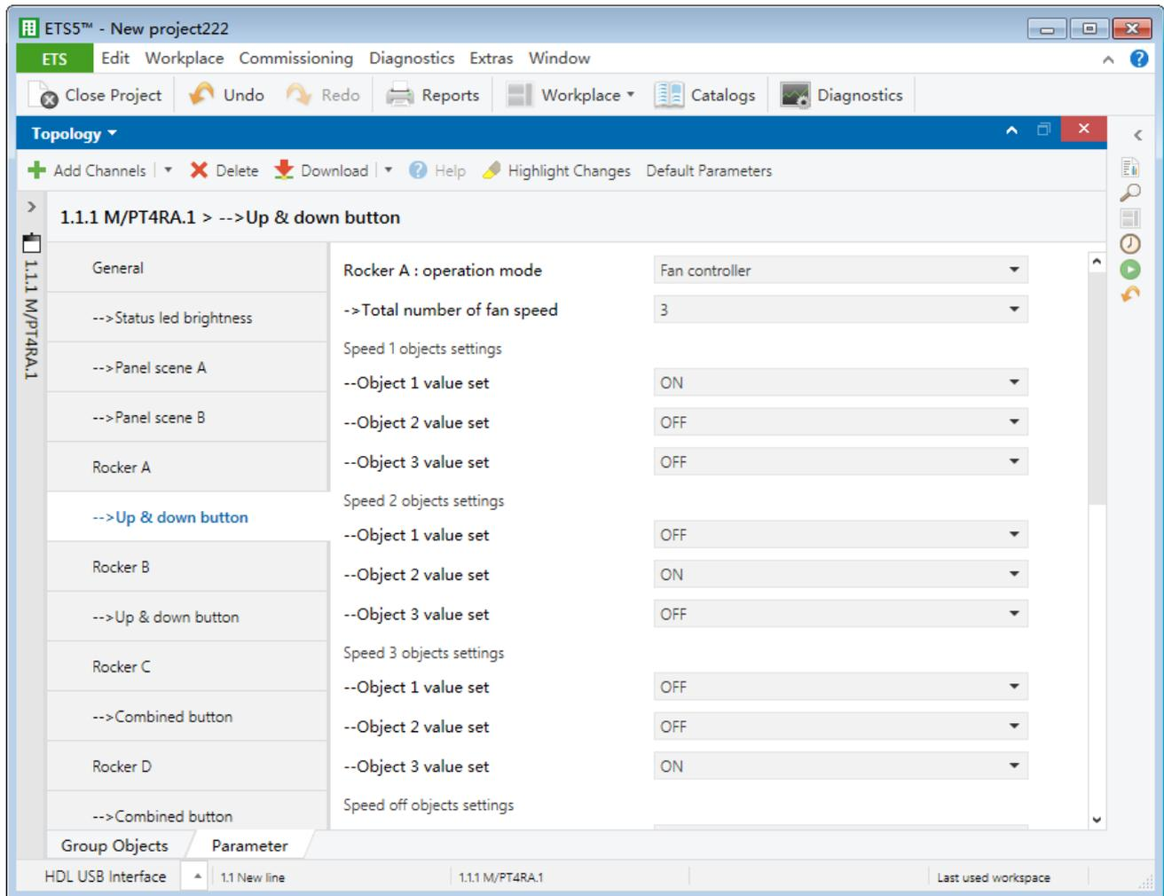
**Figure 3-28 Fan controller setting**
