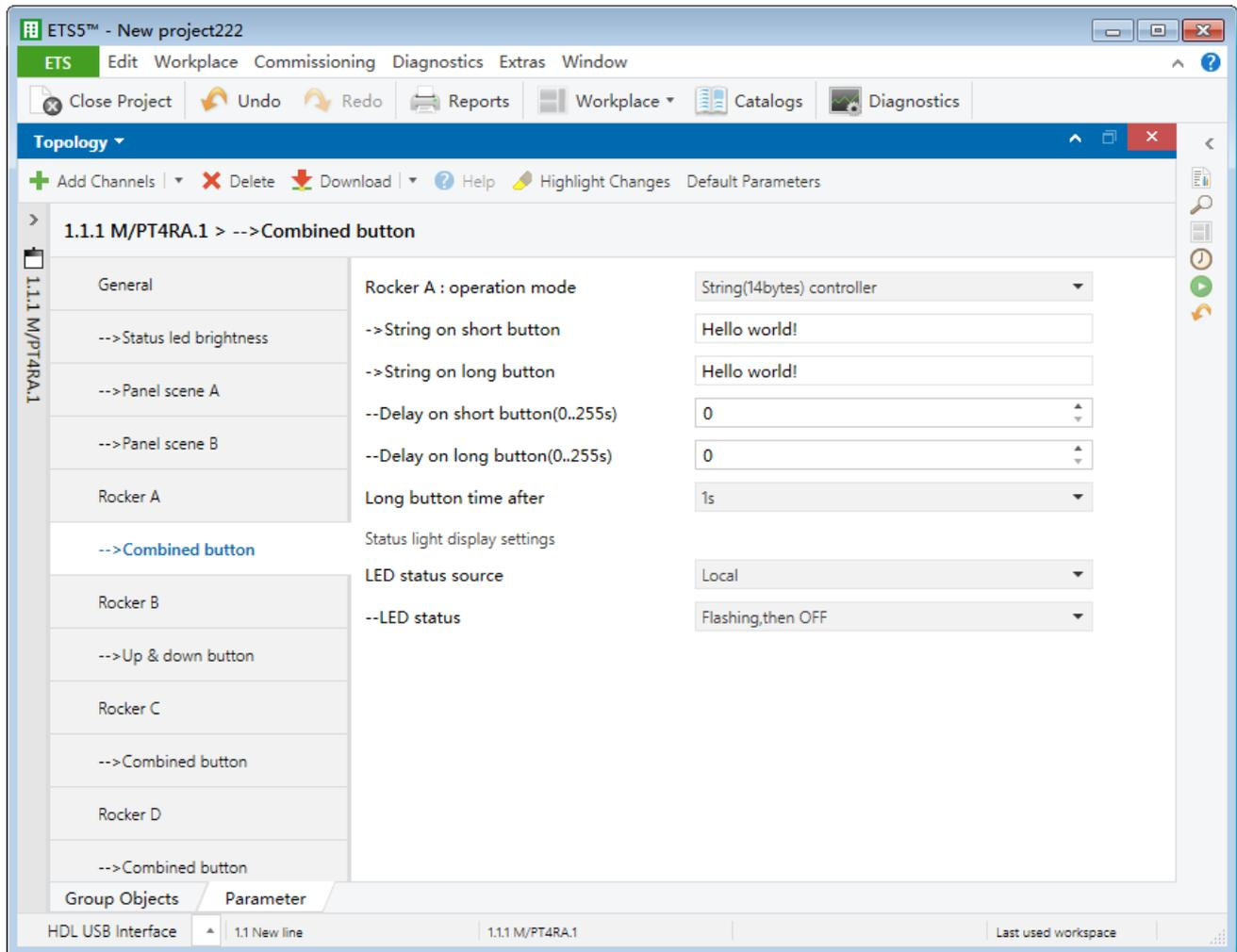
**Figure 3-11 14-byte string controller setting**
