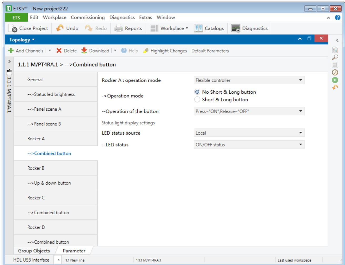
**Figure 3-6 Flexible controller setting**
