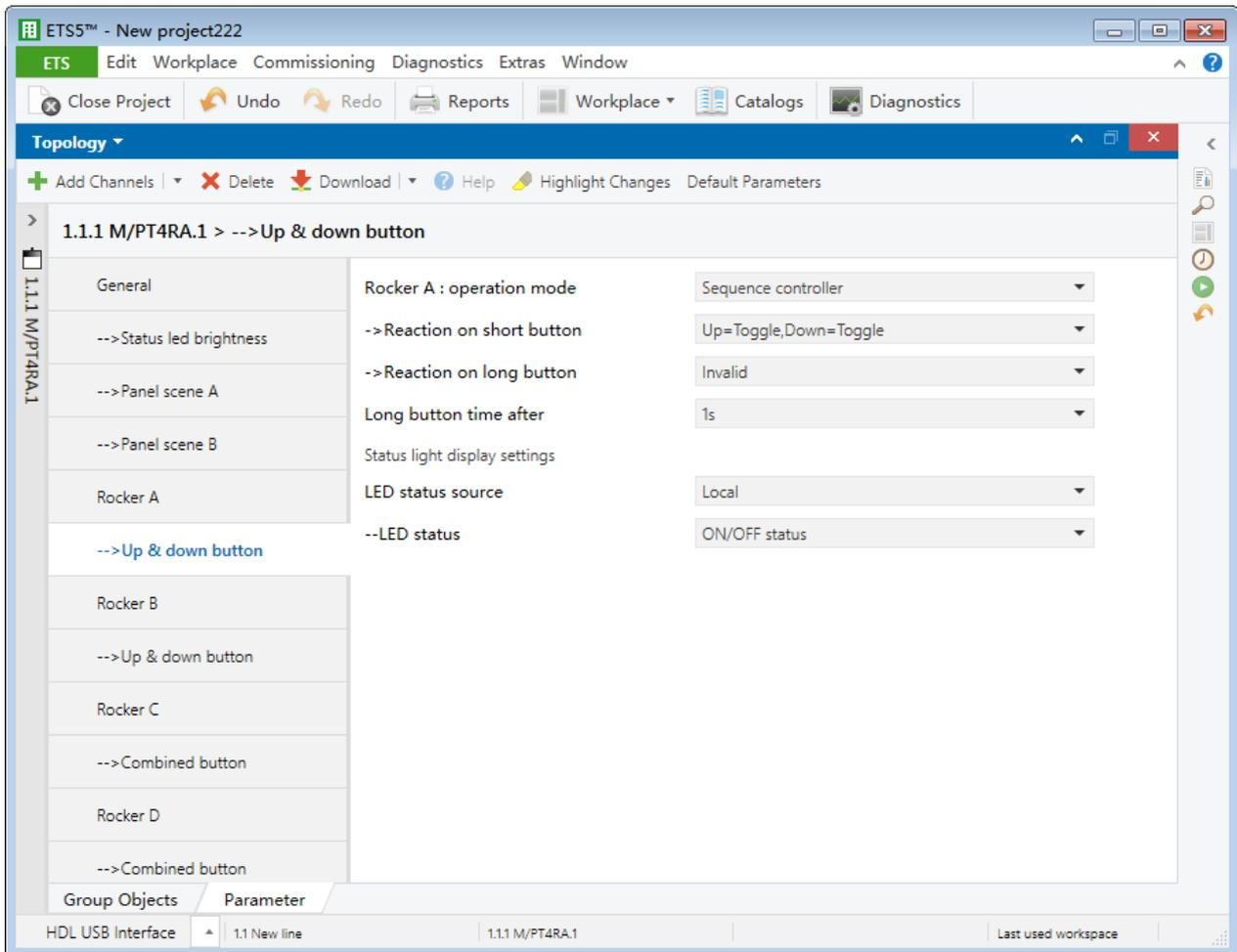
**Figure 3-22 Sequence controller setting**
