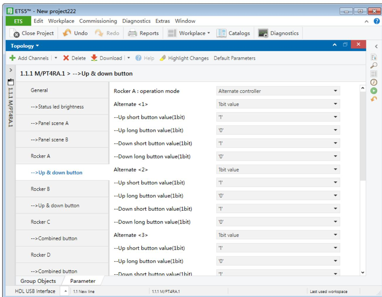
Figure 3-26 Alternate controller setting
