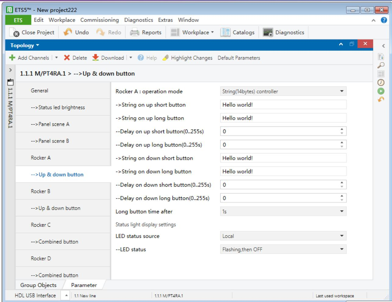
**Figure 3-25 14-byte string controller setting**
