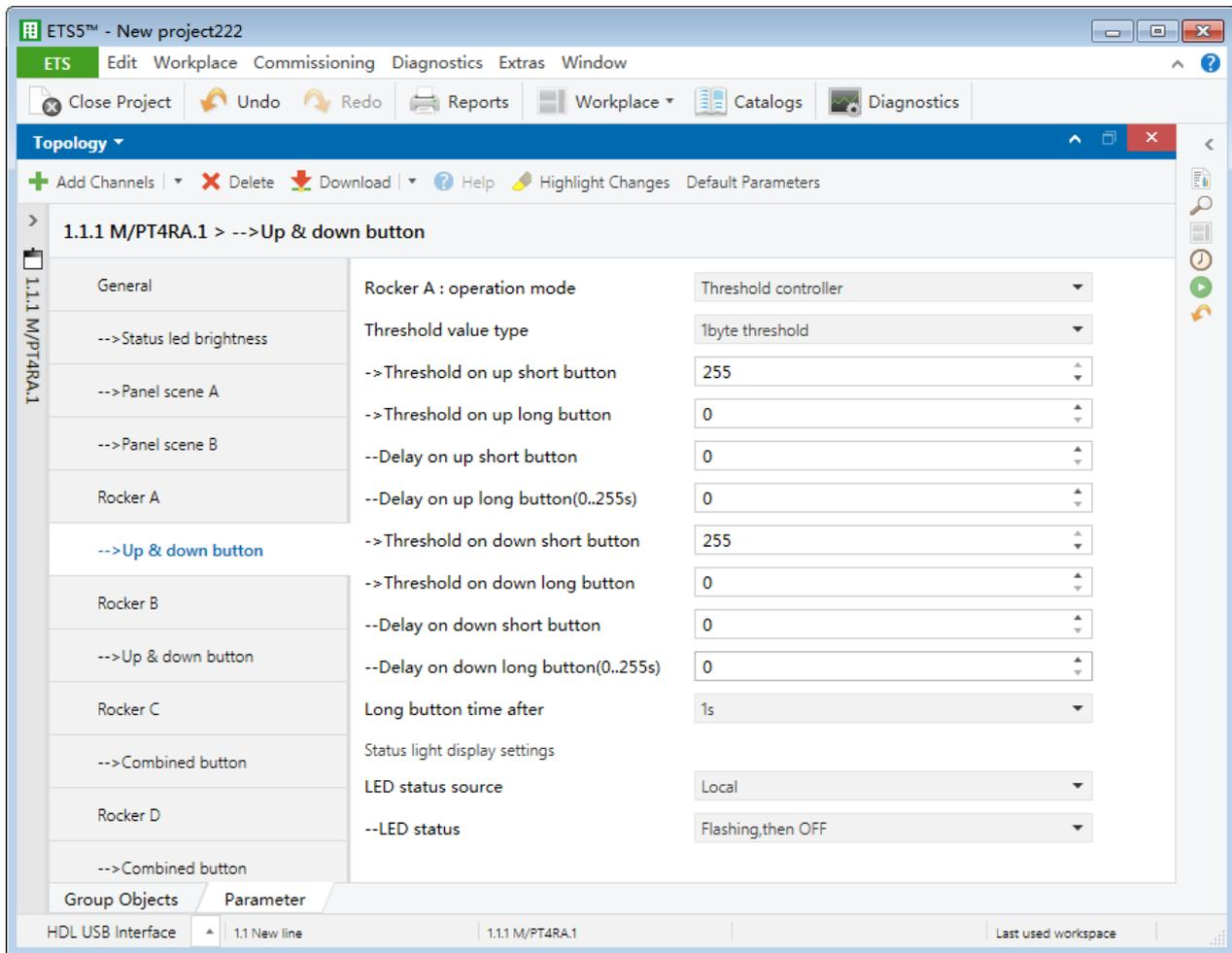
**Figure 3-24 Threshold controller setting**
