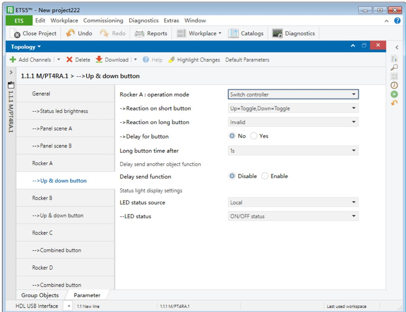
**Figure 3-17 Switch controller setting**
