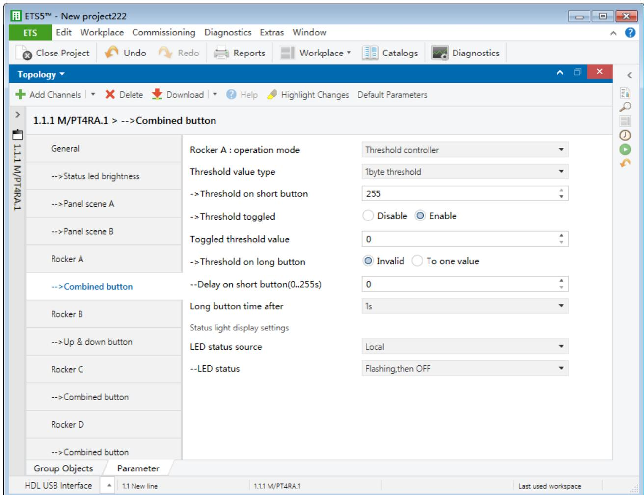
**Figure 3-10 Threshold controller setting**
