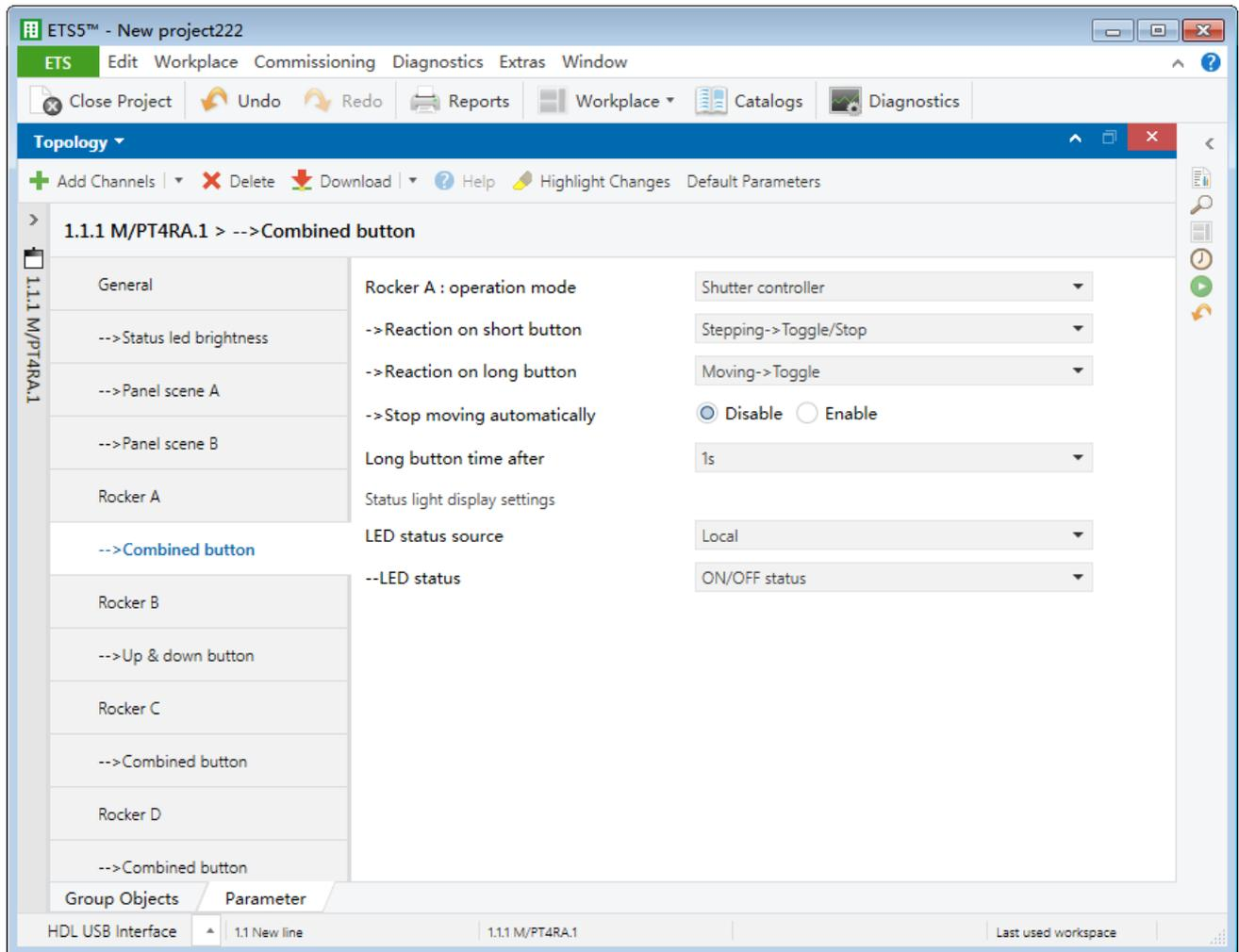
**Figure 3-5 Shutter controller setting**
