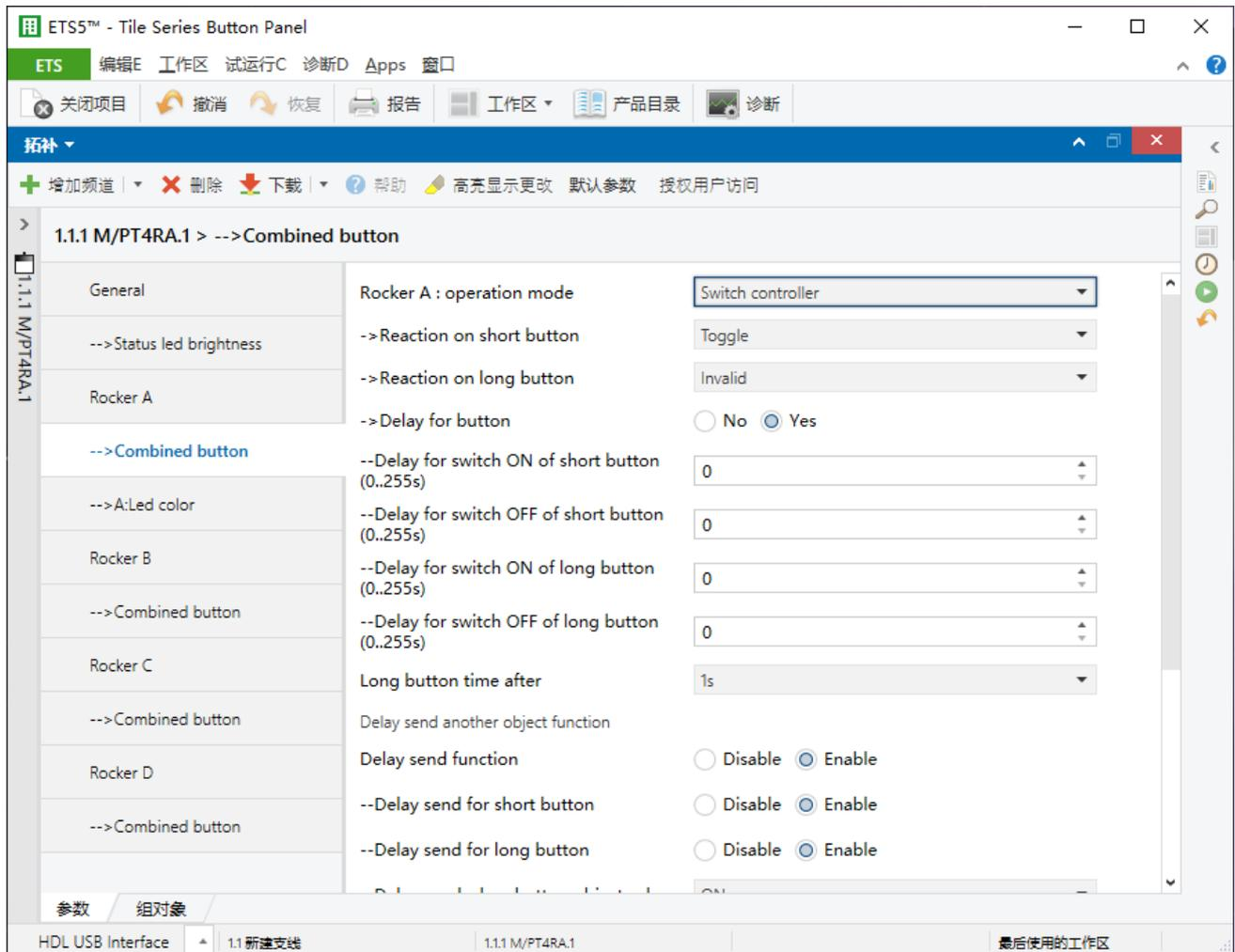
**Figure 3-3 Switch controller setting**
