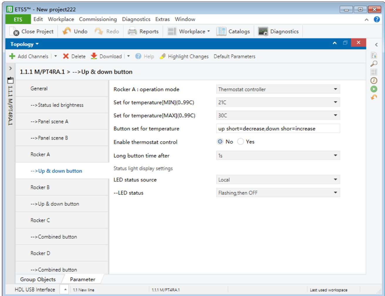
**Figure 3-29 Thermostat controller setting**
