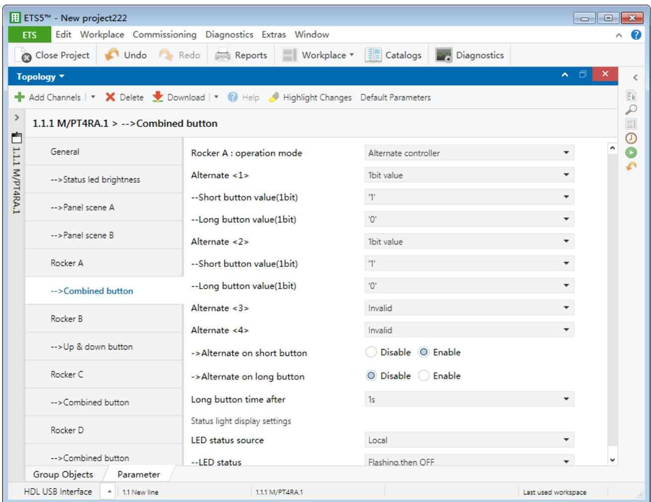
Figure 3-12 Alternate controller setting
