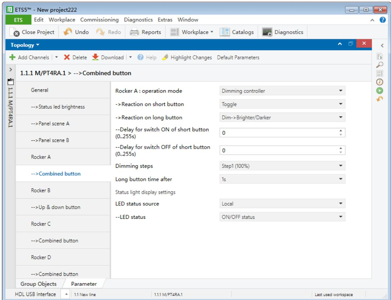
**Figure 3-4 Dimming controller setting**
