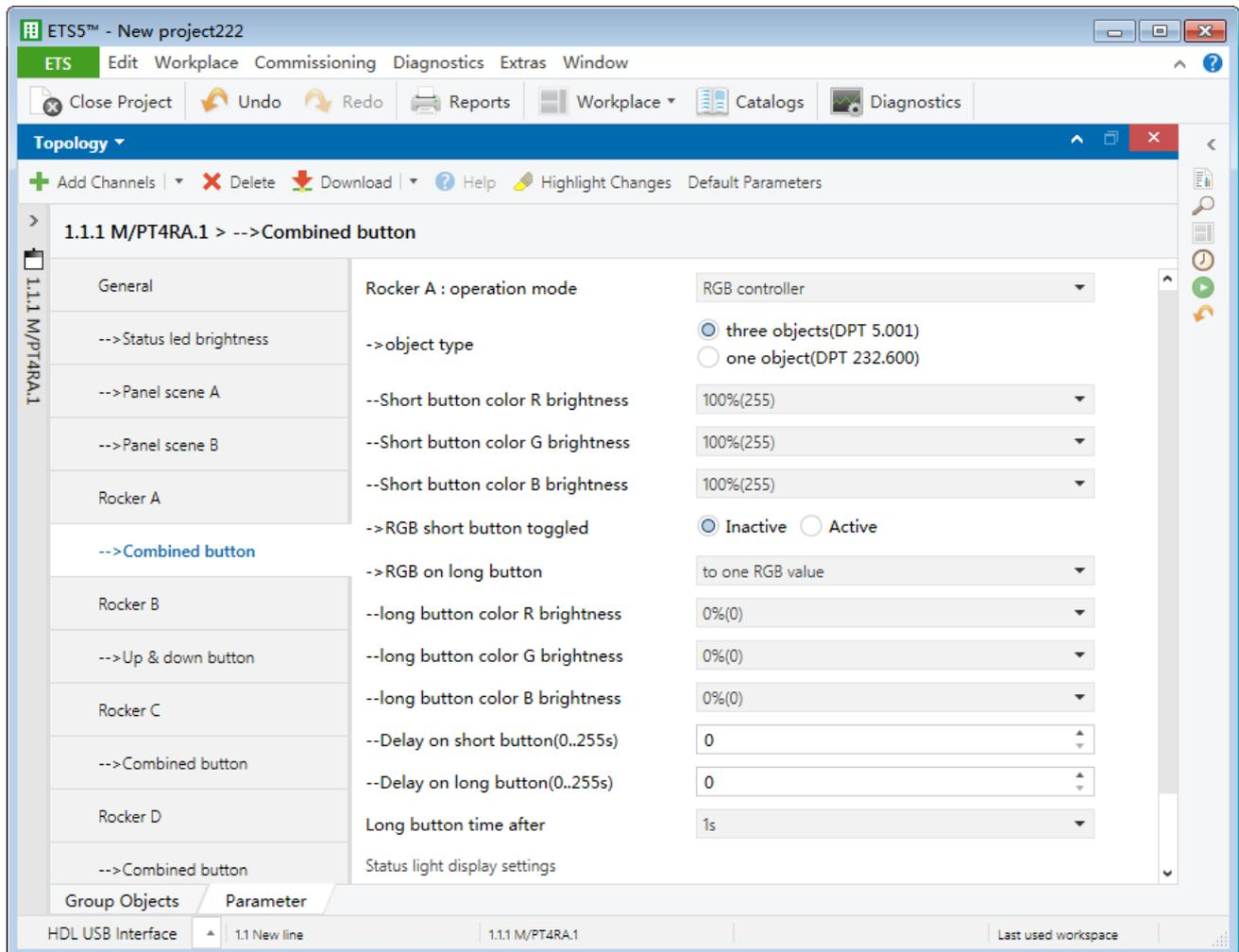
**Figure 3-13 RGB controller setting**
