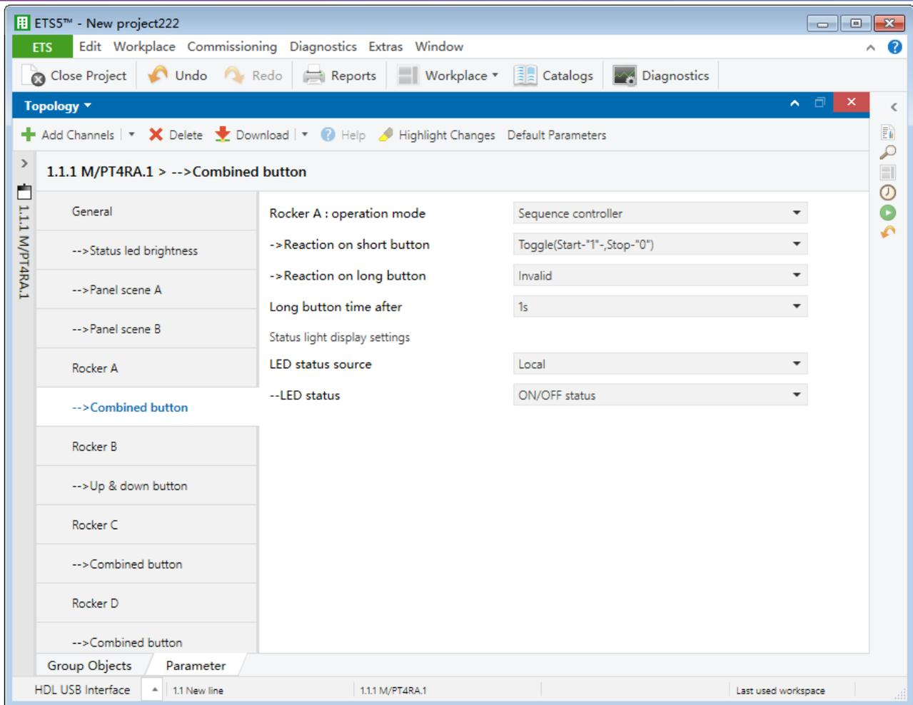
**Figure 3-8 Sequence controller setting**
