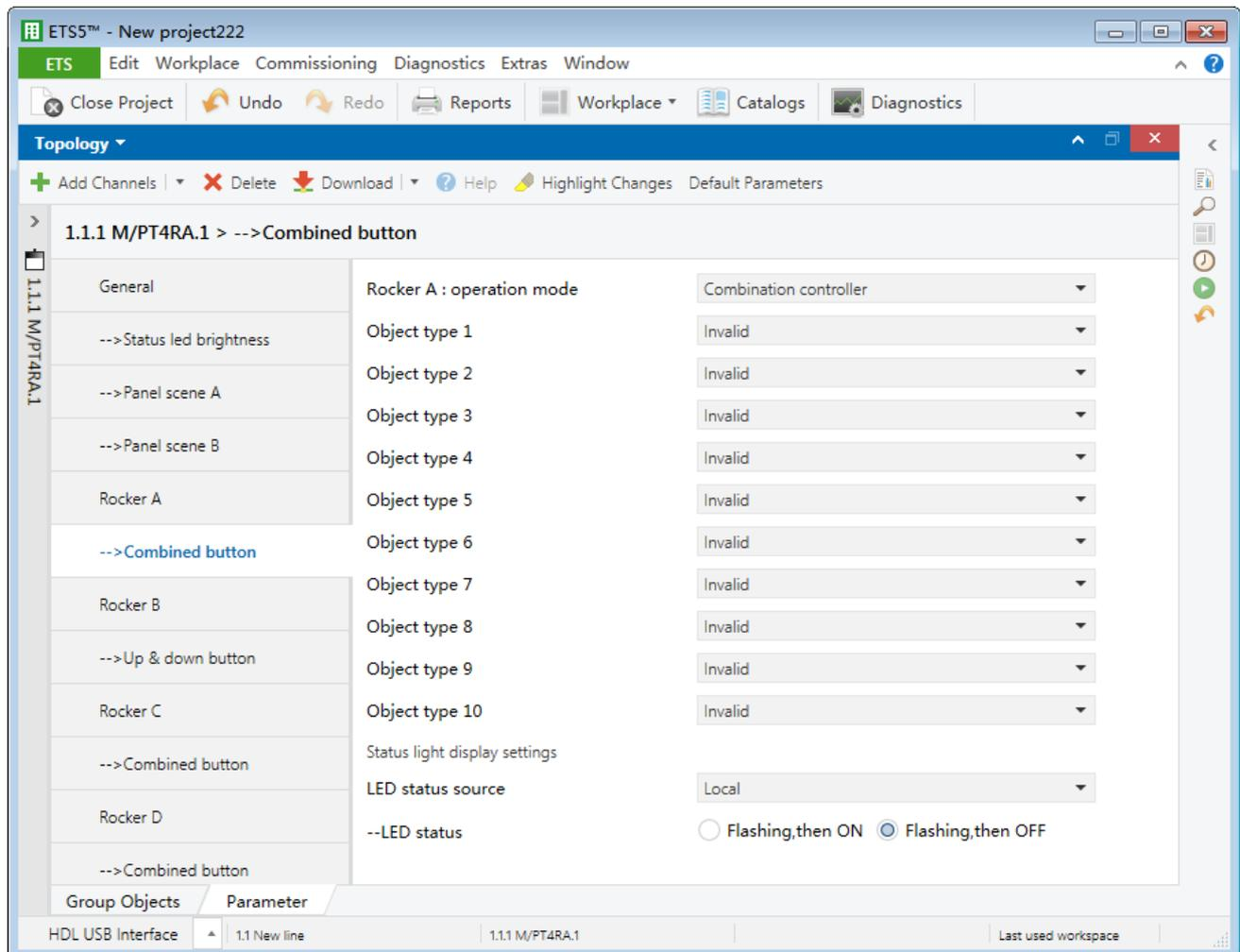
Figure 3-15 Combination controller setting
