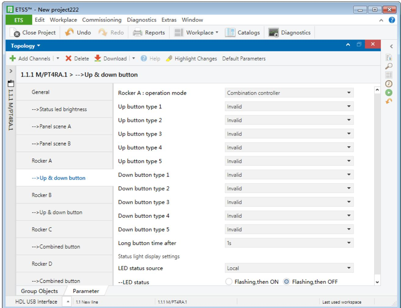
Figure 3-30 Combination controller setting
