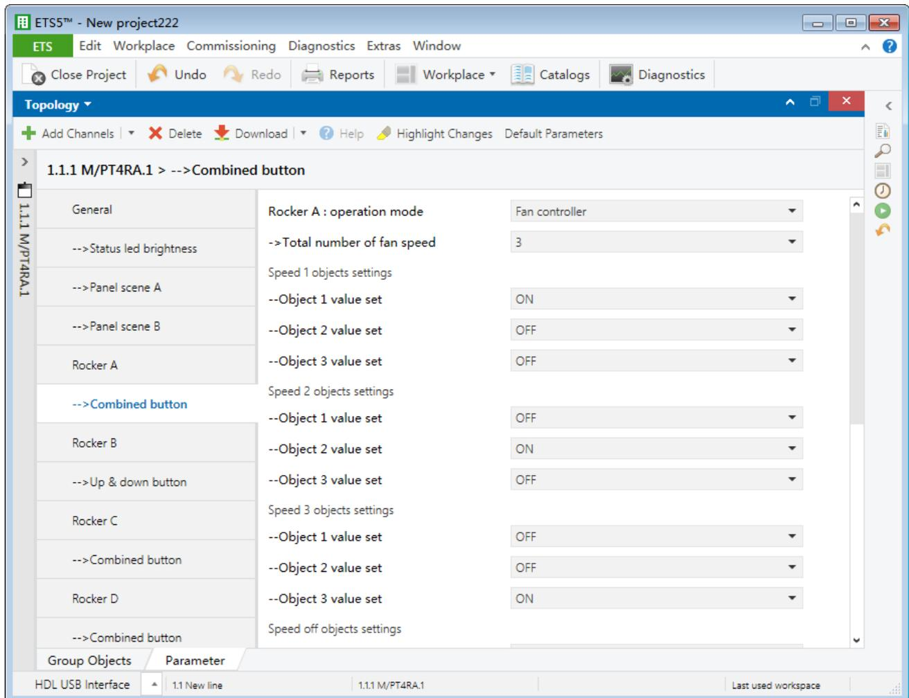
**Figure 3-14 Fan controller setting**
