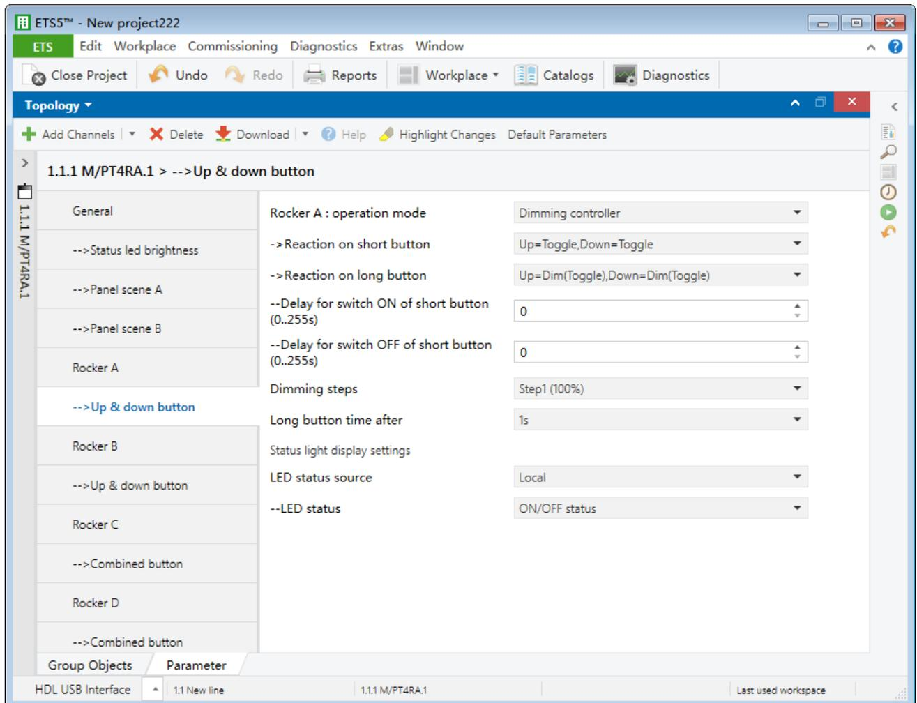
**Figure 3-18 Dimming controller setting**
