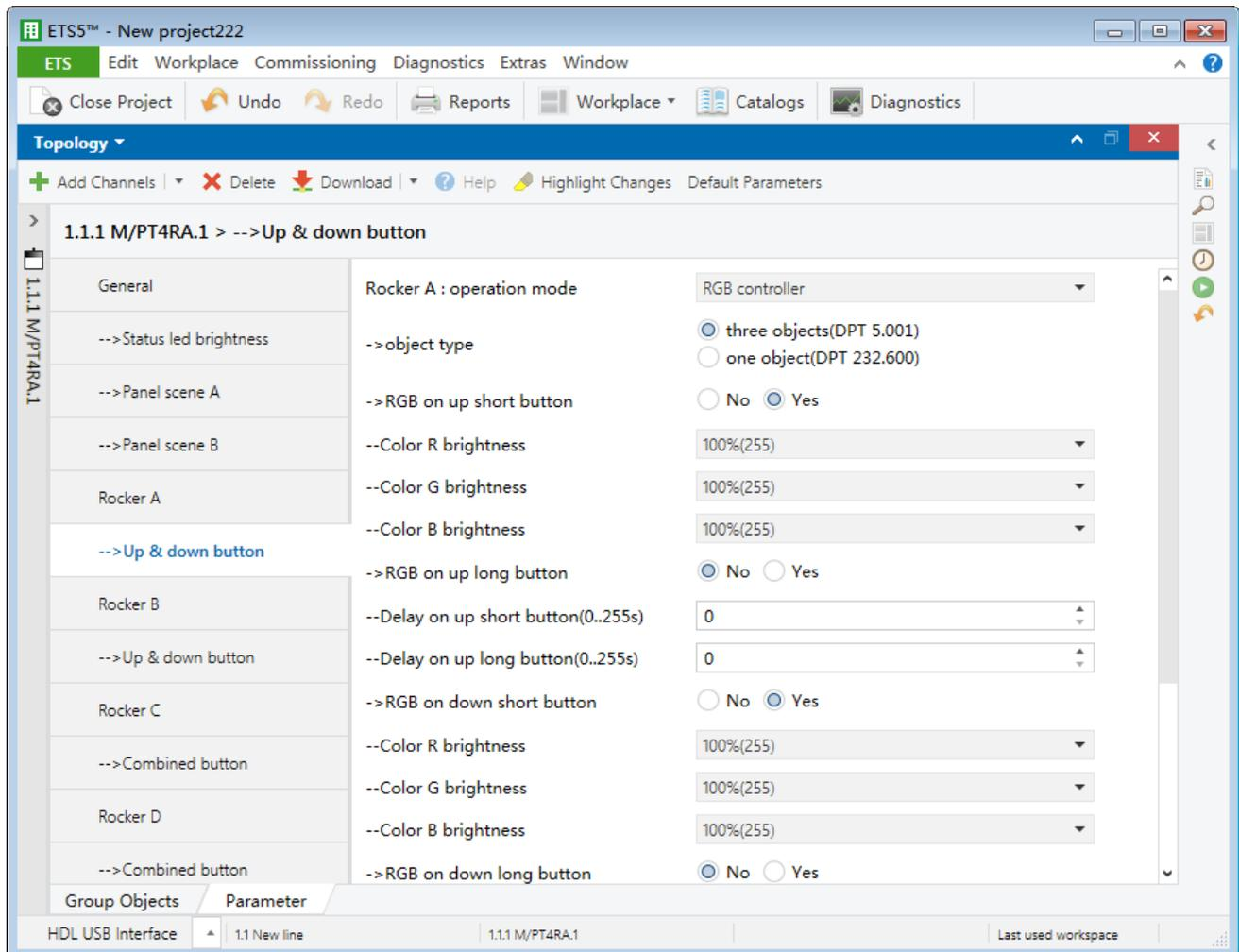
**Figure 3-27 RGB controller setting**
