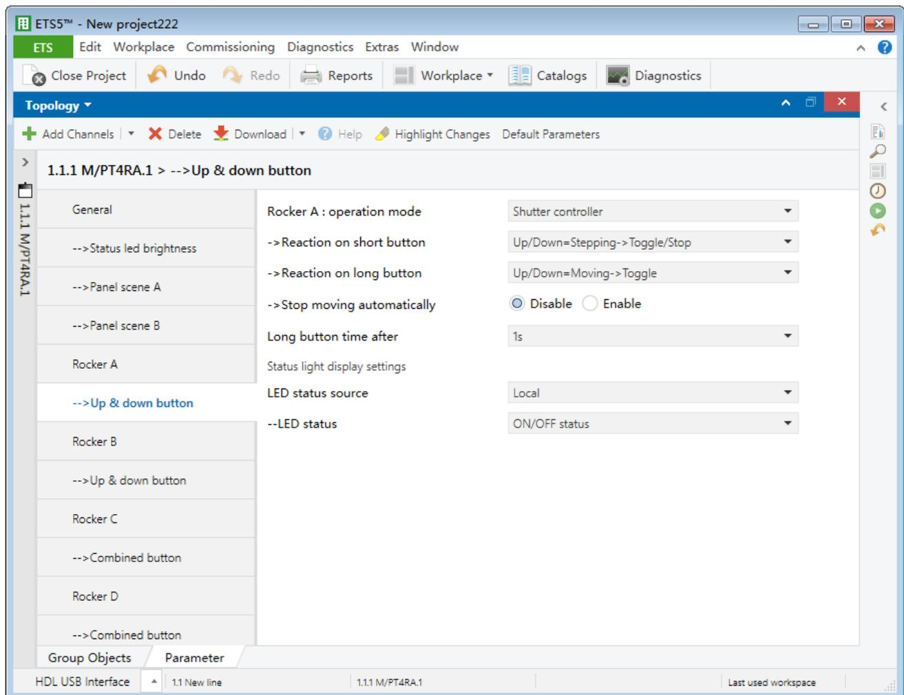
**Figure 3-19 Shutter controller setting**
