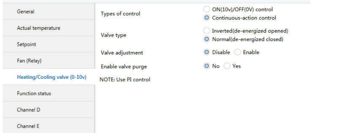
The screenshot shows a configuration window for 'Heating/Cooling valve (0-10v)'. On the left, there are tabs for 'General', 'Actual temperature', 'Setpoint', 'Fan (Relay)', 'Heating/Cooling valve (0-10v)', 'Function status', 'Channel D', and 'Channel E'. The 'Heating/Cooling valve (0-10v)' tab is active, showing the following settings:
