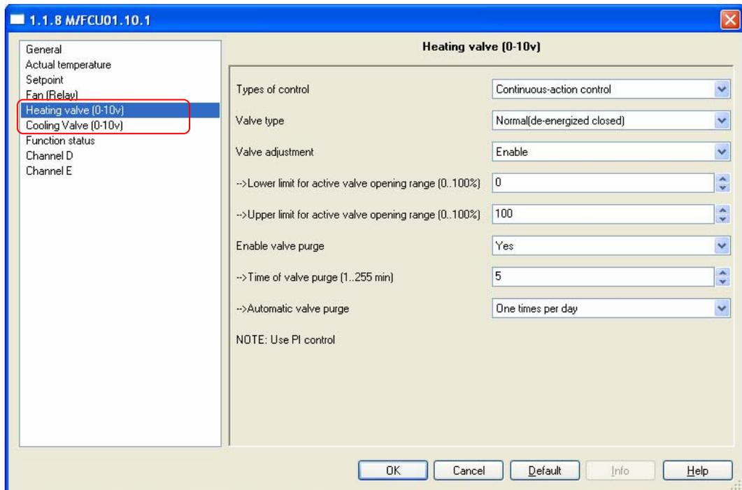
Fig.25: “Heating valve (0-10v)” parameter window
