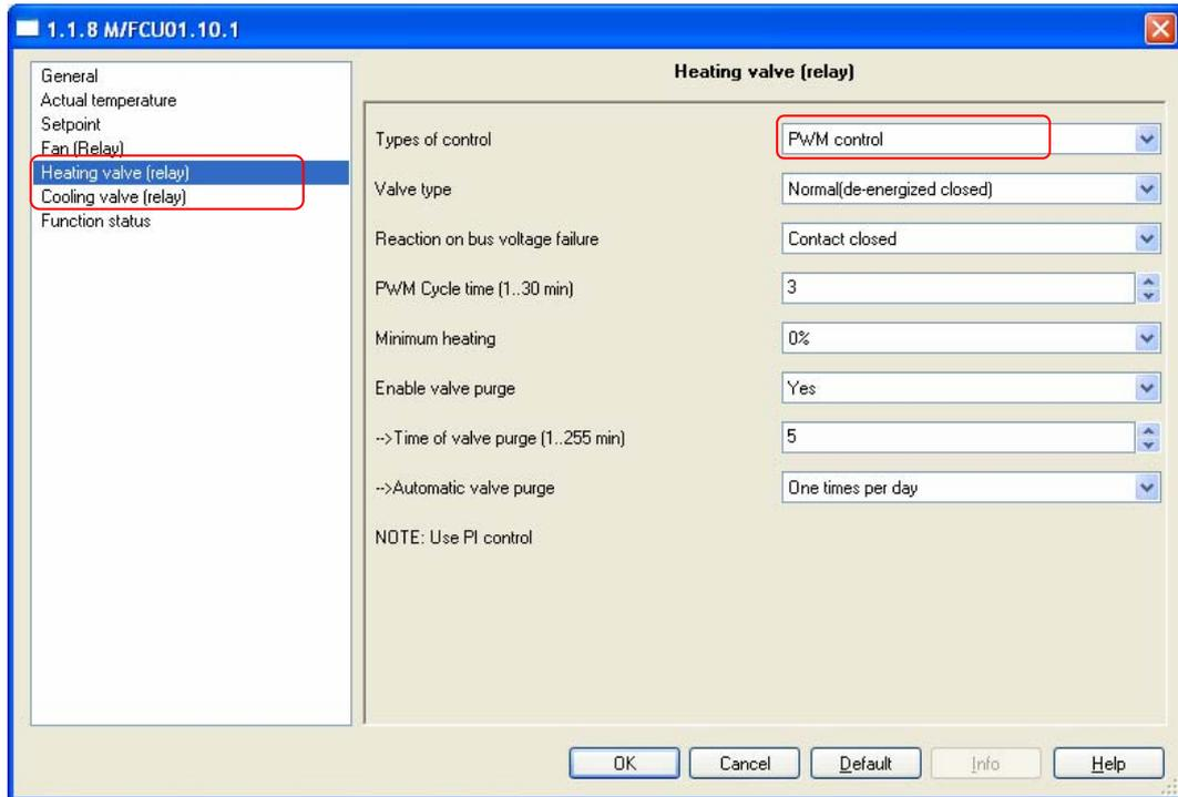
Fig.22: “Heating valve (relay)” PWM control parameter window
