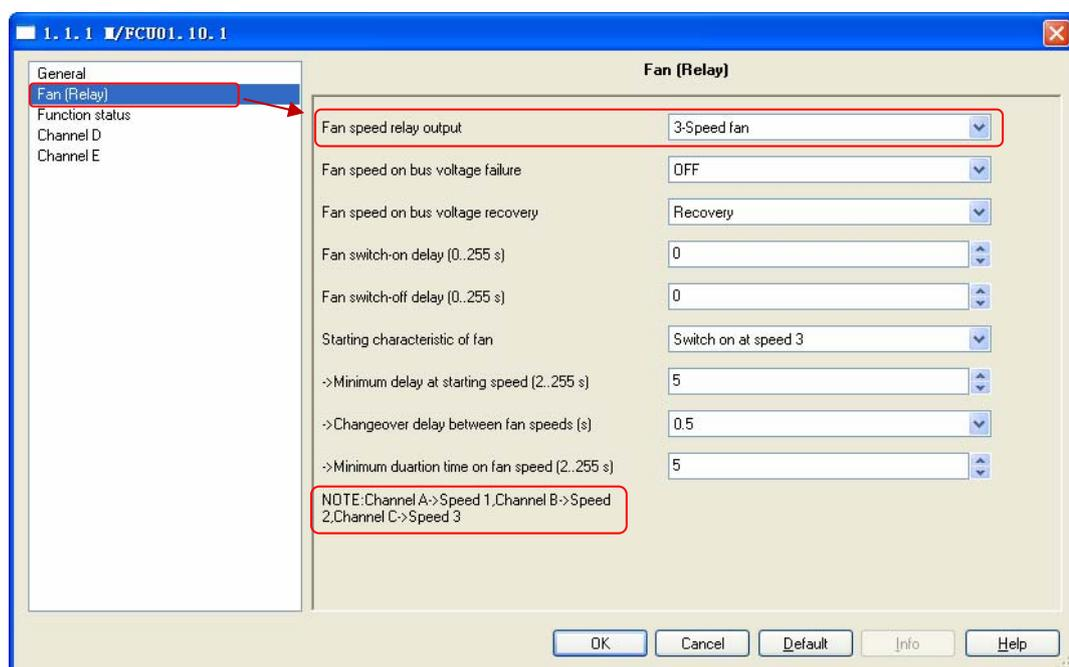
Fig.12: “Fan(relay)” parameter window
