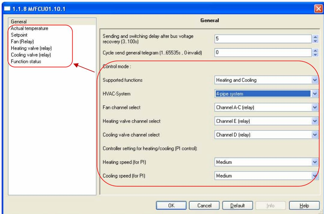
Fig.3: “Heating and Cooling” 4-pipe system parameter window
