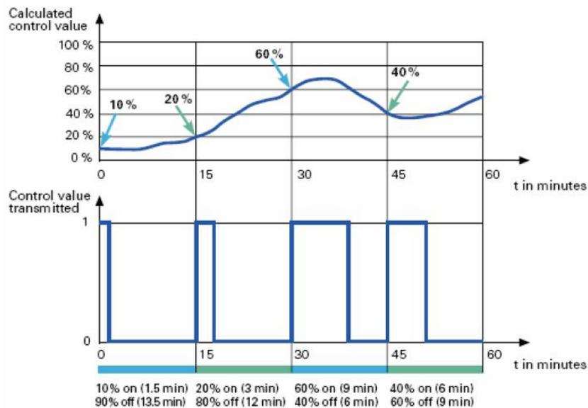
Fig.19: PWM control diagram
