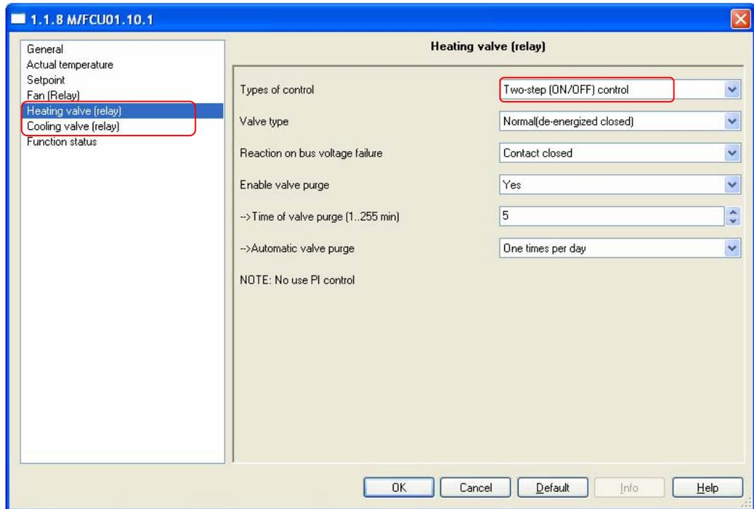
Fig.17: “Heating valve (relay)” *Two-step(ON/OFF) control* parameter window
