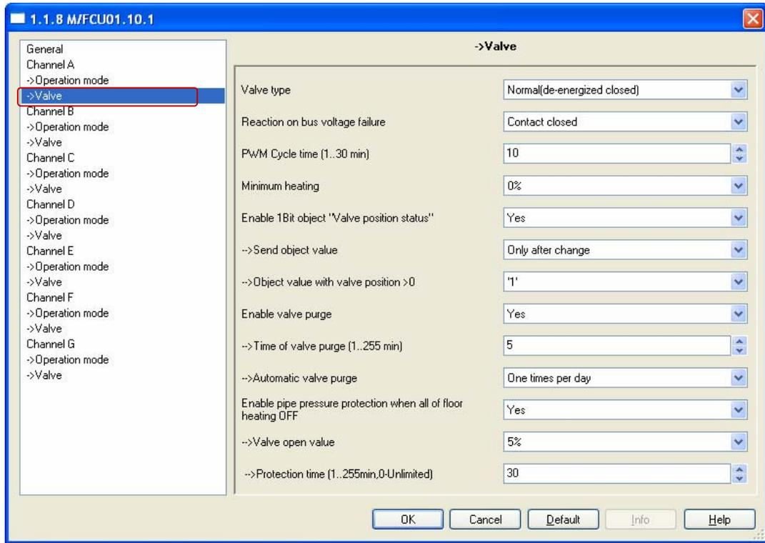
Fig.39: "Valve" floor heating parameter window
