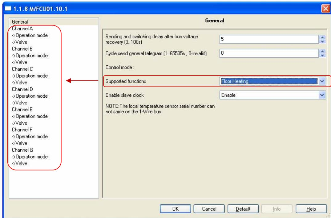
Fig.33: “Floor Heating” parameter window
