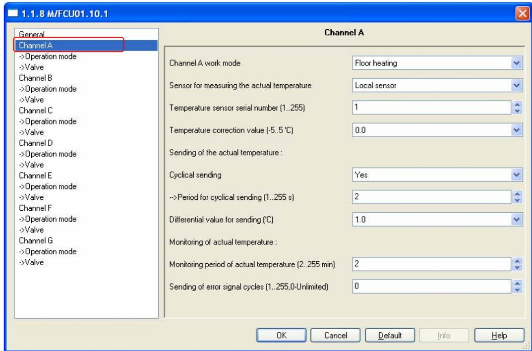
Fig.34: “Channel A” floor heating parameter window
