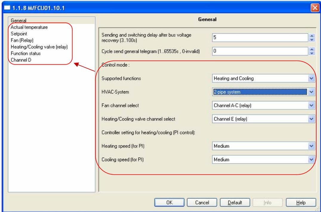
Fig.2: “Heating and Cooling” 2-pipe system parameter window
