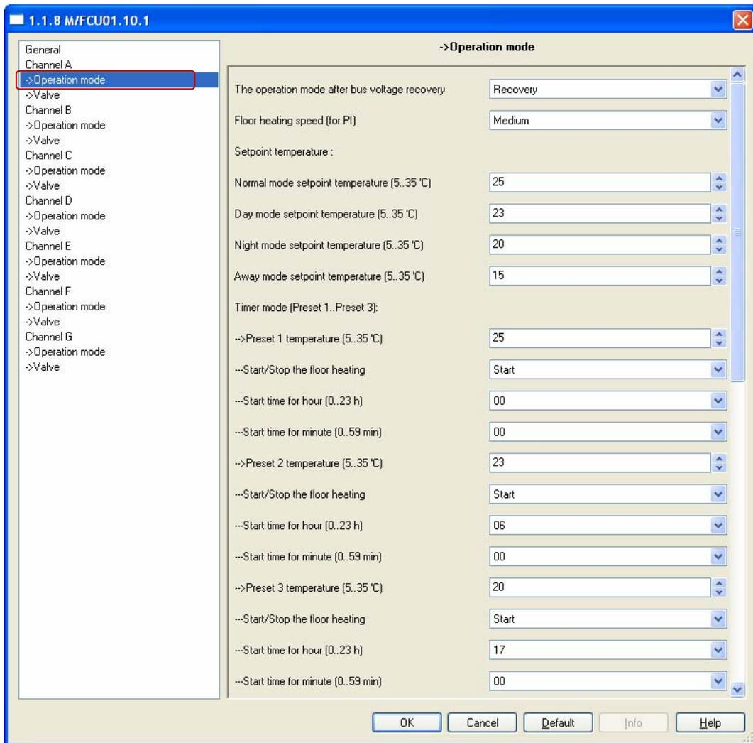
Fig.37: “Operation mode” floor heating parameter window
