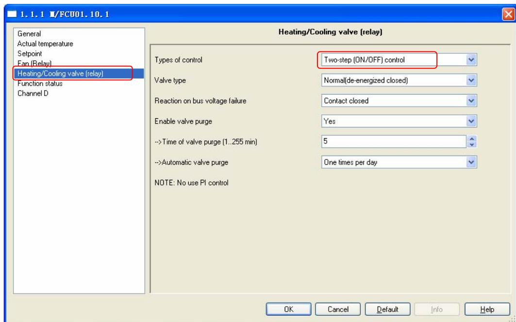
Fig.16: “Heating/Cooling valve (relay)” *Two-step(ON/OFF) control* parameter window
