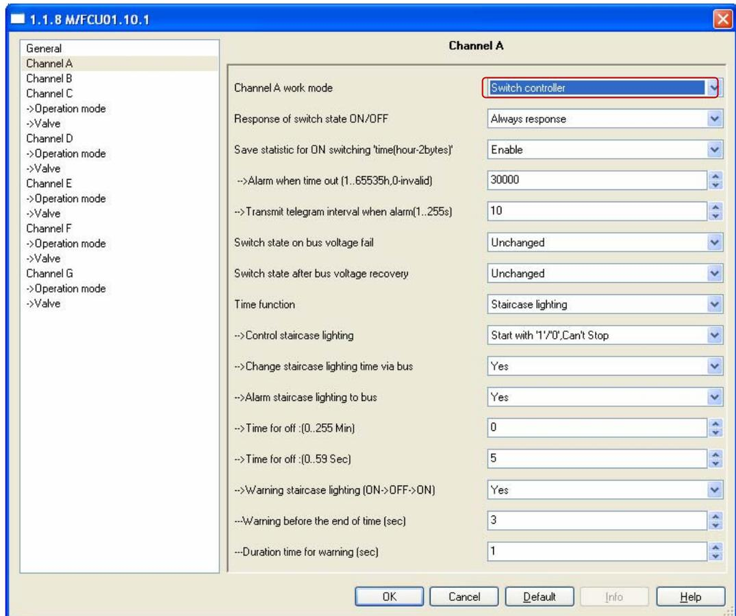
Fig.42: “Channel A work mode of switch controller” parameter window
