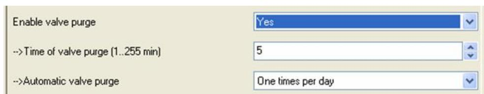
Fig.26: Enable valve purge
