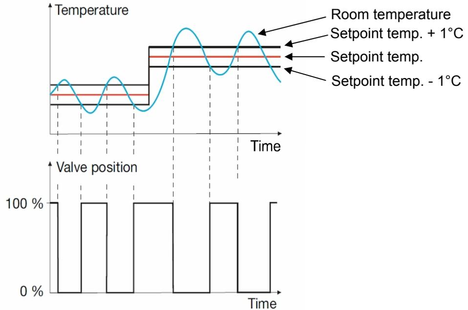
Fig.18: Diagram for 2-step control
