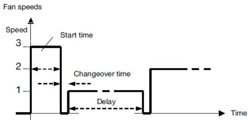
Fig.14: Switch fan on at speed 3
