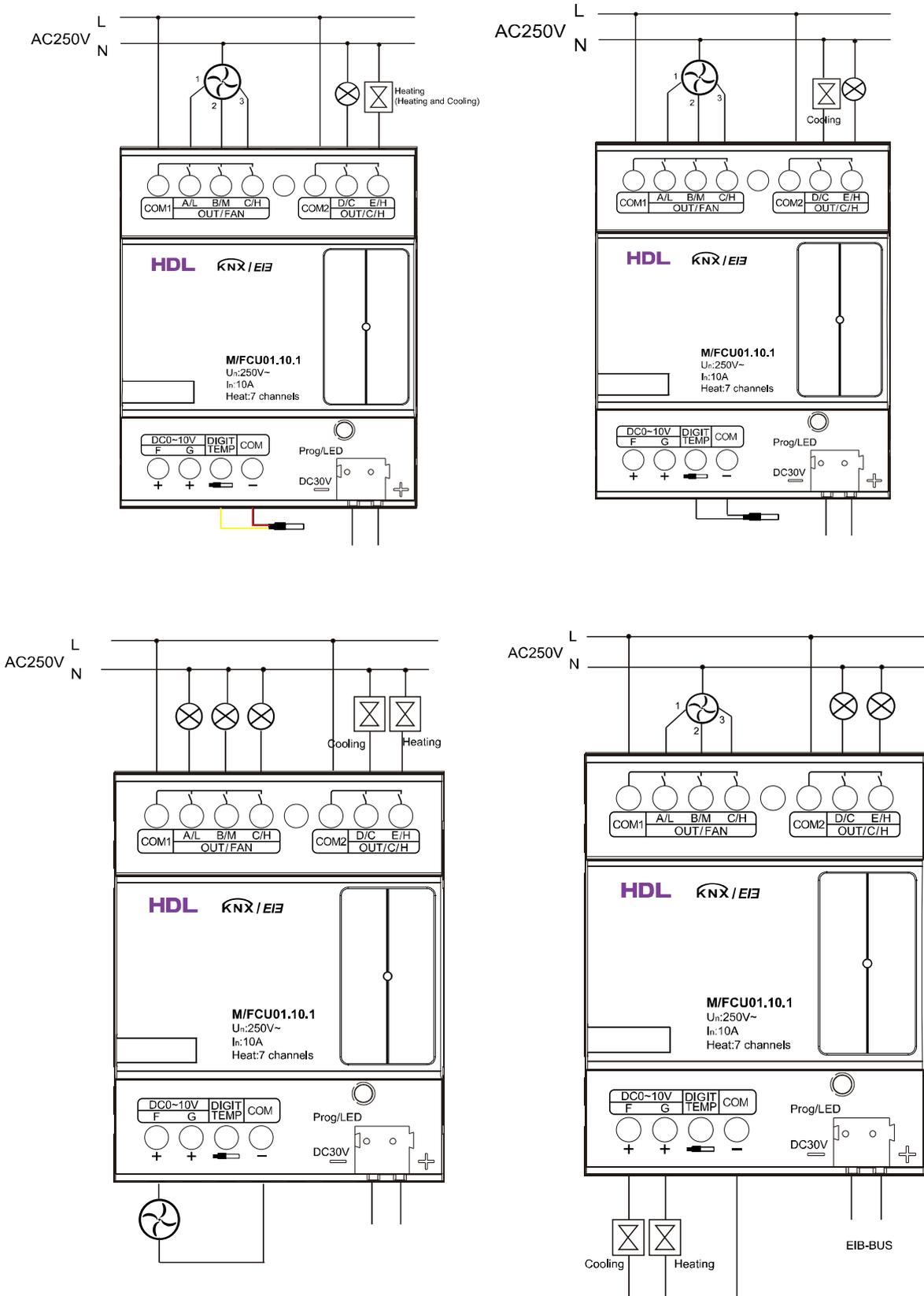
2、 Floor heating and switch actuators:
