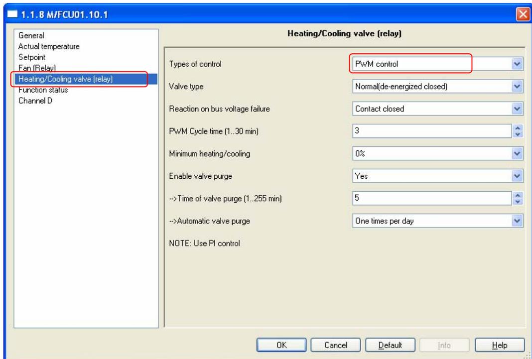
Fig.21: "Heating/Cooling valve (relay)" PWM control parameter window
