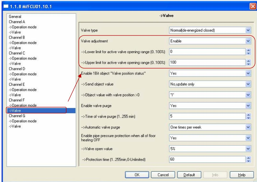
Fig.41: “Valve” floor heating channel F,G parameter window
