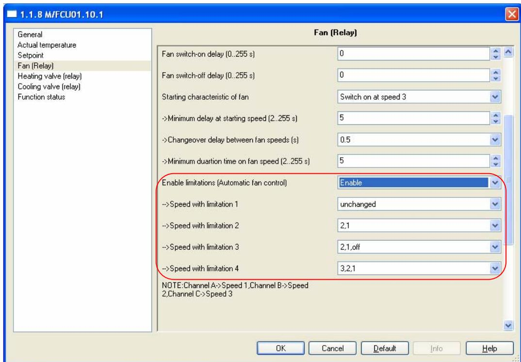
Fig.15: Enable limitations (Automatic fan control)
