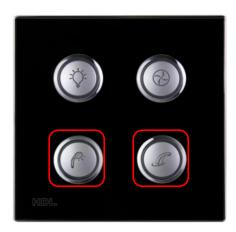
About the wireless DLP panel, power off the device, press these two buttons at the same time, shown as below, power on.
