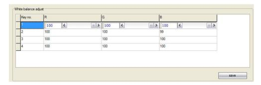
For some panels, the displaying LED color has little difference from the one you set, user can adjust its white color with this function. After adjusted, all colors can be indicated correctly.
