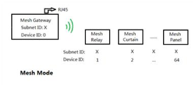
Note: Subnet ID X and Y are different, Gateway has the fixed Device ID 0.
