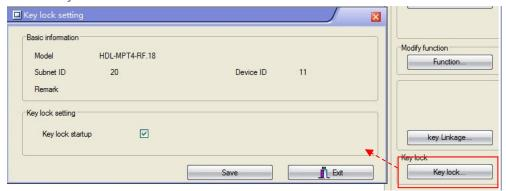
Enable/disable all the keys. When tick this option, all the keys cannot send out any control commands, it's locked.
