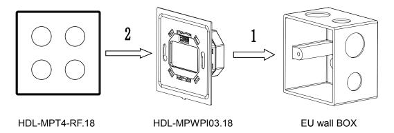
Separation: Use a screwdriver with 2.5mm insert to split gap, pry up, from position 1 to position 2, the wiring hole will open. Then separate the panel and power interface.
