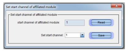
C. Set the start channel, if the channel is to be used in conjunction with the HDL-MHRCU.433 module, it is recommended that the start channel is set as 1. If an affiliated module like the SB-DN-RMIX20 is to be used then set the start channel as 23 or >23, because the Mix control channels occupied channel 1 to 21 of host module,
