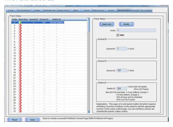
To shield (disable) a panel button when a scene is in use, the buttons information must be entered into the panel setup window.
