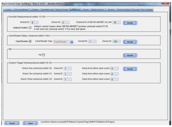
**Doorbell Setup:** Input the doorbell panel subnet ID, device ID, and channel ID. Then assign a channel to the bell. If the bell is connected to the "doorbell channel", (see Section "1.3 Description and Wiring of the HDL-MHRCU.433" for details), channel 22 must be assigned to the bell.
