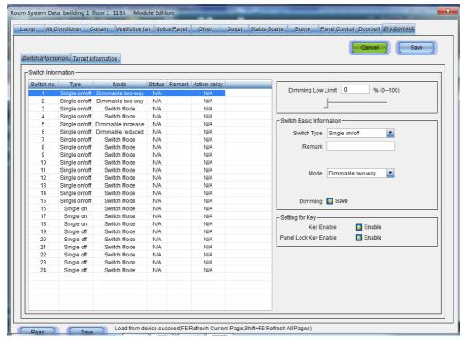
The HDL-MHRCU.433 has 24 dry contacts, which can be connected to ordinary switches. This enables the HDL host module to be used in conjunction with ordinary switches.
