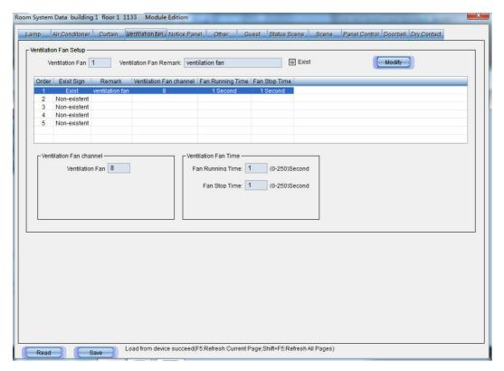
The HDL-MHRCU.433 supports up to 5 ventilation fans, each fan must be assigned a single channel from the HDL-MHRCU.433.
