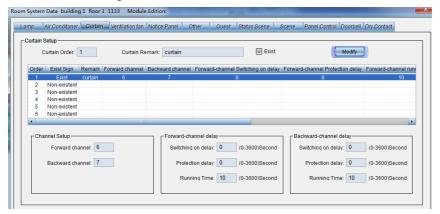
4) Add Ventilation fan: Assign channel 8 to the fan.
