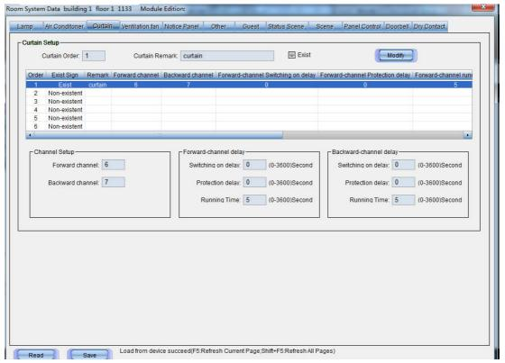
The HDL-MHRCU.433 supports up to 6 curtain motors, each curtain motor needs to be assigned 2 channels from the HDL-MHRCU.433. One channel is used for forwards, and the other channel being is used for backwards.
