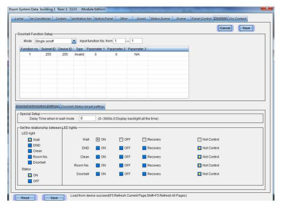
When a 3<sup>rd</sup> party standard doorbell panel is used, its information can be entered into the doorbell tab, and enabling its status to be shown.
