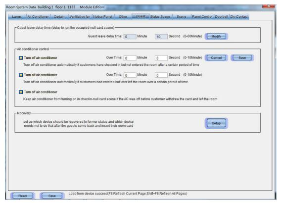
**Guest leave delay time:** When a guest removes their keycard from the card reader, a delay time can be programmed. This enables the HDL-MHRCU.433 to activate the *occupied-null* card scene after a set time has elapsed.
