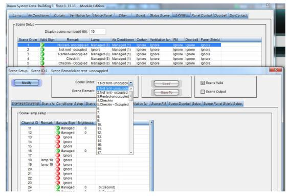
The system allows up to 99 scenes to be created, in these scenes lamps, air conditioners, curtains, fans, radios, and panels can be configured. (To use "Scene Panel Shield Setup", the 'Panel Control Tab' must first be set up).
