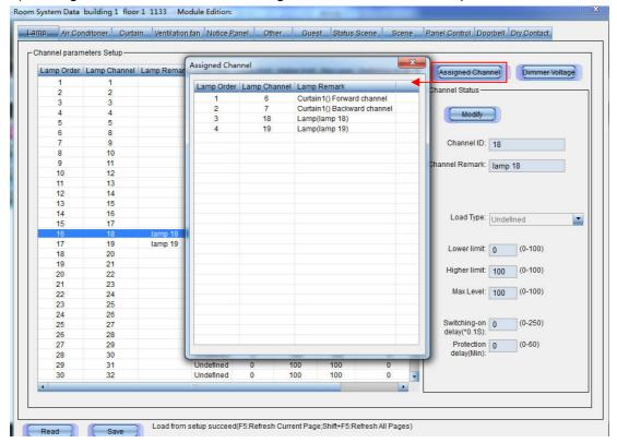
Dimmer Voltage: The dimming voltage can be selected.
