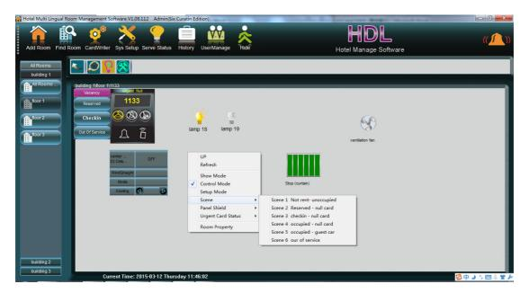
Using control mode, all the configured devices and appliances in a room can be managed. The Scene/Panel Shield/Urgent Card Status, can also be simulated.
