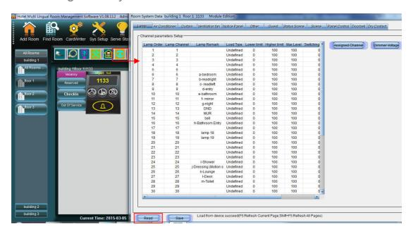
The elements that make up a room such as doorbell panel, curtains, lights, fans and A/C etc., can be set in the room system data window.
