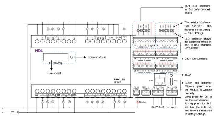
If the HDL-MHRCU.433 is to be used in conjunction with another module, connect the additional module to the "INNER-BUS" port of HDL-MHRCU.433.
