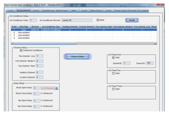
The HDL-MHRCU.433 supports up to 4 air conditioners, each AC can be controlled by up to 3 AC Panels (thermostats).
