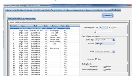
Switch 1 – Controls the bedside light; the host module subnet ID is 1, the device ID is 33, and channel 18 is connected to the bedside light.
