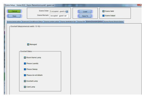
The status of the HDL doorbell can be managed in each scene, in scene 5 (occupied-guest card), the room name lamp, doorbell lamp, and the card lamp have been set as on.
