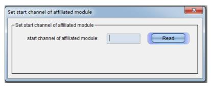
B. Then press the 'PROG' button on the affiliated module until the LED indicator turns red. After this then click on 'Read', and the below window will then appear. (If you wish to change the Mix control's default start channel, you must press the 'PROG' button on the HDL-MHRCU.433.)
