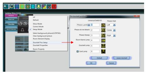
Please refer to the process shown in step 5. If indirect control is not selected, universal switches 1 to 6 can be sent to the doorbell panel. This can enable the triggering of laundry/DND/sweep/room name/doorbell/card lamp.
