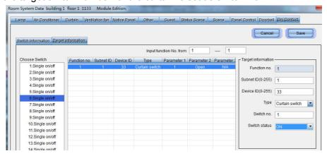
Switch 10 - Is used for the guest check out process, the host module subnet ID is 1, and the device ID is 33. When the host module receives 'universal switch no.2 on' command, it signifies that the guest wants to check-out.
