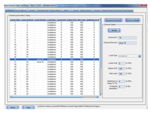
The HDL-MHRCU.433 has 48 control channels and 21 Mix control channels, the first mix control channel is channel 1. (For further information, please refer to section "7.5 Set Start Channel of Affiliated Module".)
