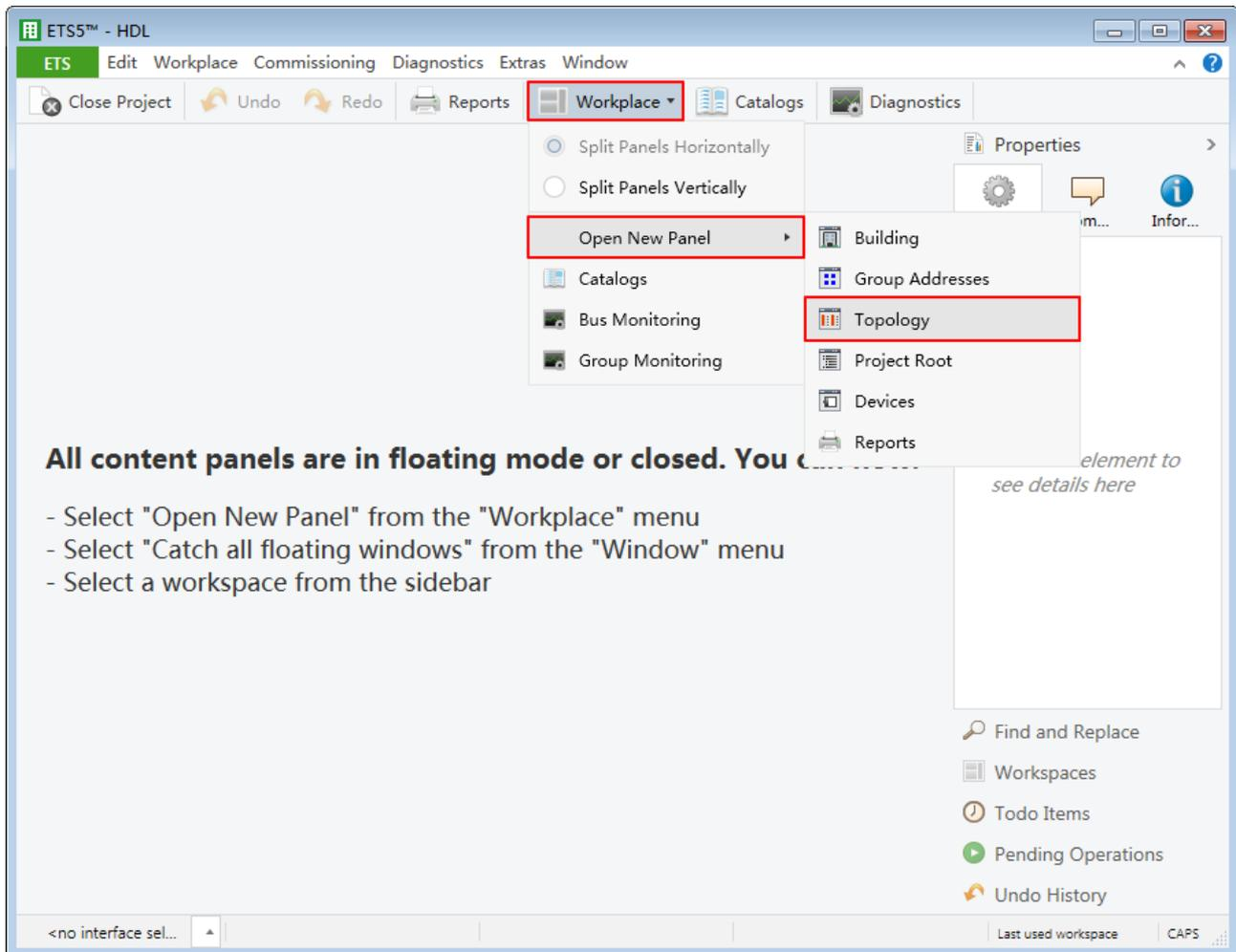
Figure 1-7 Open configuration window
