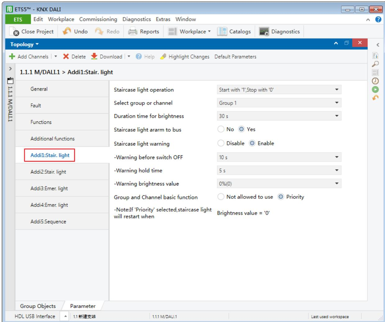
Figure 8-2 Staircase light setting
