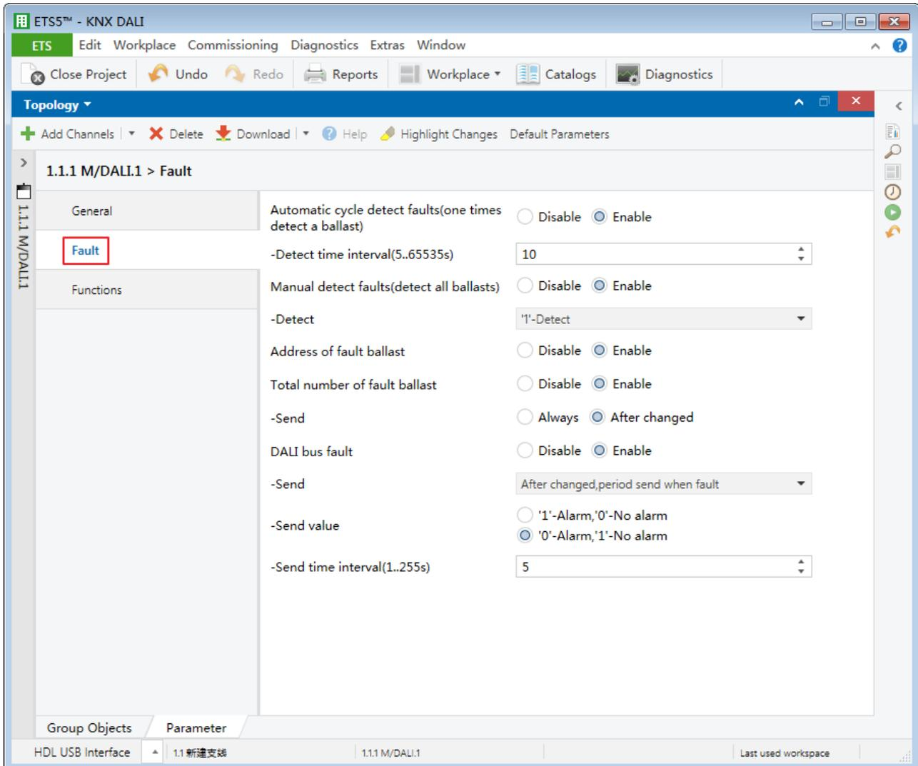
Figure 2-2 Fault detection
