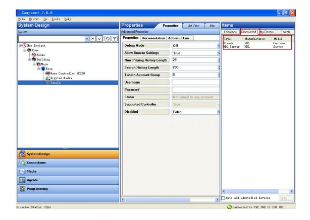
Double click the device, will be added to the current project. Right click the device, you can read the device information, such as subnet ID, device ID...
