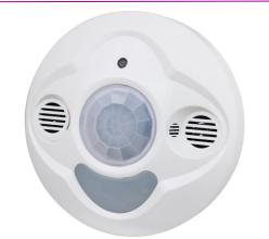
HDL-MS12.2C 12 in 1 sensor includes temperature sensor, PIR motion sensor, LUX sensor ,ultrasonic sensor, dry contacts, IR received, IR emitter, 2channel 5A relay output and logic block. The logic block can combine all sensors for different applications. It supports HDL security mode and command.
