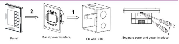
Installation: Hold the edge of the panel (shown as above), insert the power interface module vertically. Do not push the panel too hard.
