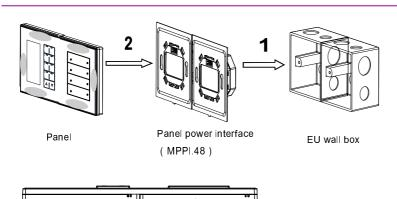
Installation: Hold the edge of panel, (see pictures on the left) ,insert the power interface module vertically.
