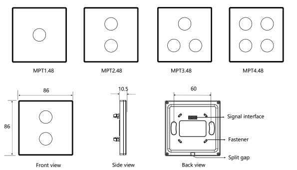
Touch button function: On/off, dimming
