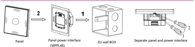
**Installation:** Hold the edge of panel (shown as above), insert the power interface module vertically. Do not push the panel too hard.
