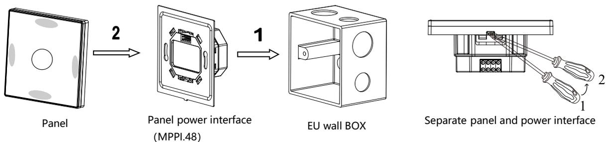
**Installation:** Hold the edge of panel (shown as above), insert the power interface module vertically. Do not push the panel too hard.
