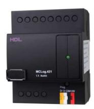
HDL-MCLog.431 is the HDL Logic Module. It has 960 Logic blocks, and the inputs condition of logic can be set scene status, channel status, date, week, time, external input value, external input status etc. By using different logic relations to set up different control target. 4 Logic relations are available for each logic block: AND, OR, NAND, NOR.
