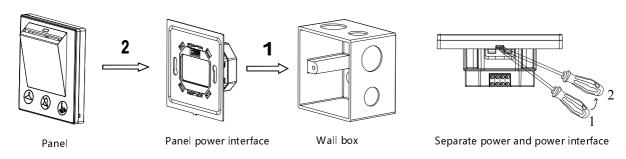
Installation: Hold the edge of panel (shown as above), insert the power interface module vertically. Do not push this module too hard. Split: Insert a 2.5mm screwdriver to the split gap, pry up from position 1 to 2, wiring hole will open. Then separate the panel and power
