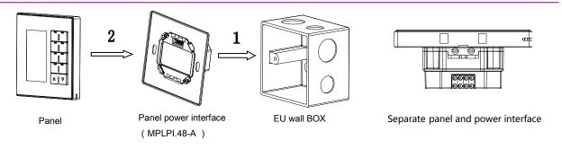
Installation: Hold the edge of panel, insert the power interface module vertically. Do not push the panel too hard.
