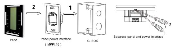
Installation: Held the edge of panel (shown as above grey area), insert the power interface module vertically. Do not push the panel too hard.
