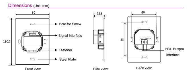
Signal Interface and fastener: They are connected with the panel switch or sensor.
