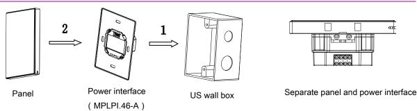
Installation: Hold the edge of panel, insert the power interface module vertically.
