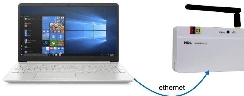
Fig.1 Wireless gateway HDL-MCIP-RF02.10 and their connection to the PC
