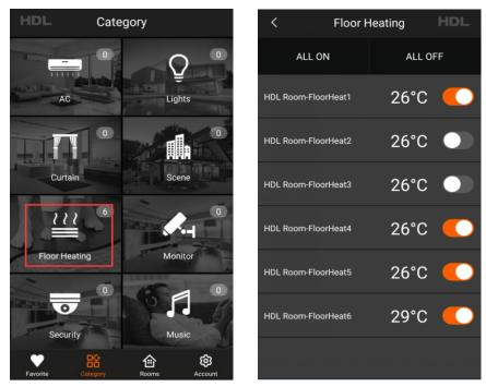
After touching the floor heating channel, we can switch the channel, set working status(e.g. floor heating, floor cooling), set working mode(e.g. day, night, normal, away and automatic), and set the temperature.
