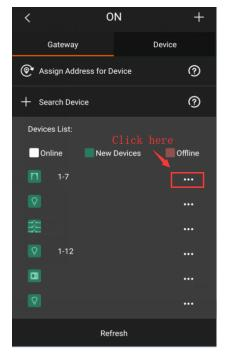
**Position:** It is used for finding out where the device is. The indicator or the channels of the device will blink for 3 times if we position it.
