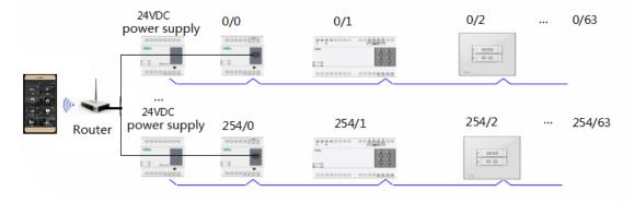
This is the basic method of controlling the HDL Buspro system by HDL ON, we can search and program the system devices by connecting the phone and the system in the same local area network (WIFI).
