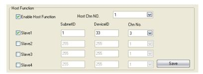
If use host function, the slave floor heating channel will synchronize with the host floor heating channel.
