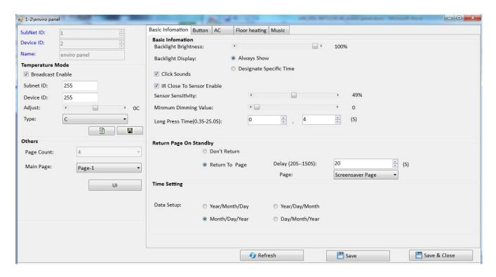
**Temperature Mode:** This panel built-in temperature sensor, can broadcast the temperature to the BUS. If the detected temperature has error, you can adjust it on the software.
