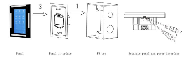
**Installation:** Hold the edge of the panel (shown as above grey area), insert the power interface module vertically. Do not push the panel too hard.
