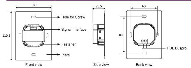
Signal Interface and fastener: To be connected with the panel switch or sensor.
