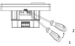
Separate the panel and the power interface
